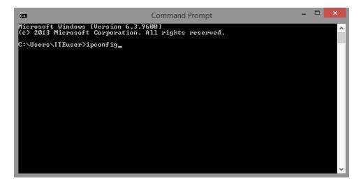
c. You will need PC 2's IPv4 Address to complete Step 5. The address can be located in the output generated from the **ipconfig** command. Under the **Ethernet adapter Local Area Connection** heading, and to the right of the **IPv4 Address** row.
